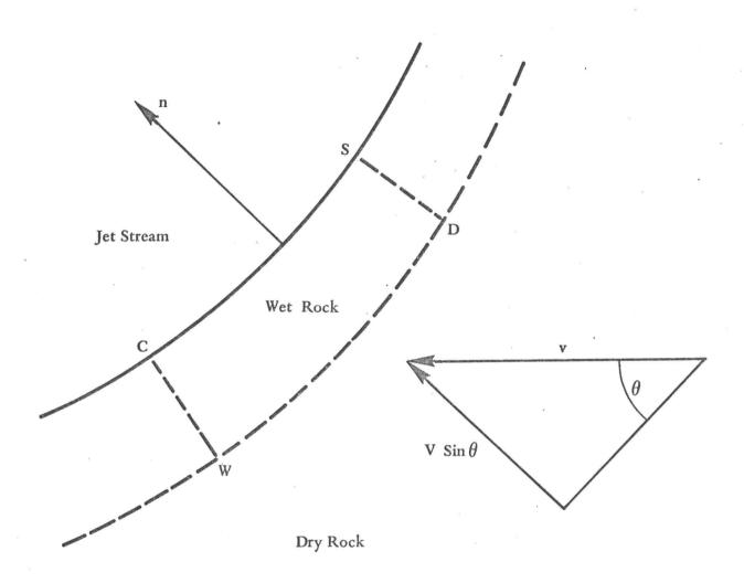
Figure 6. Permeability model. A front WD between wet and dry rock precedes the cutting surface CS.
